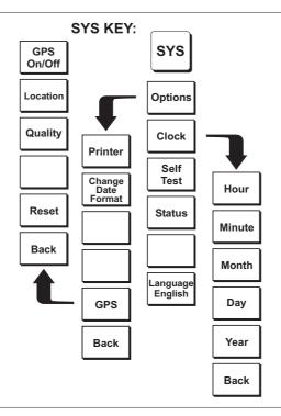
Figure 2-9. SYS Key Menu in Power Monitor Mode
