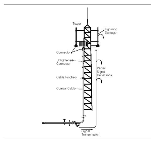
Figure 4-1. A Typical Transmission Feed Line System
