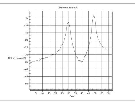
Figure B-4. Minimum Side Lobe Windowing Example
