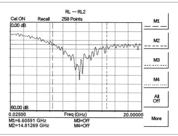
Figure 4-2. Typical System Return Loss Trace
