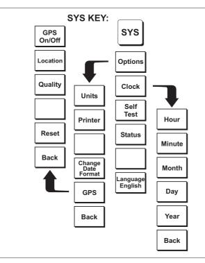
Figure 2-8. SYS Key Menu in Cable and Antenna Analyzer Mode
