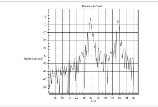
Figure B-1. Rectangular Windowing Example
