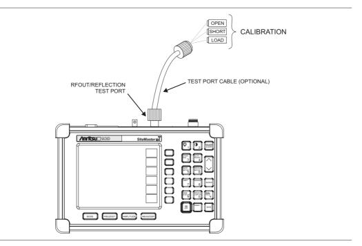
Figure 3-2. Calibration Setup
