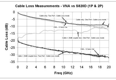
Figure 4-3. Comparison of One Port and Two Port Cable Loss Mode Measurements
