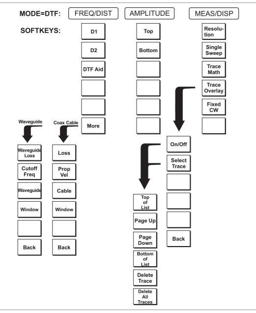
Figure 2-6. Distance to Fault Mode Soft Key Labels
