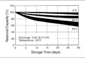
Figure 2-12. NiMH Battery Storage Characteristics
