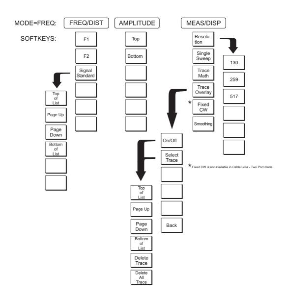
Figure 2-5. Return Loss Mode Soft Key Labels
