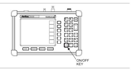
Figure 3-1. Site Master On/Off Key
