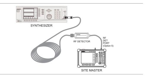
Figure 5-2. Power Monitor Measurement Setup for Thru Line Insertion Measurements
