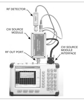
Figure 3-3. Cable Loss - Two Port Calibration Setup
