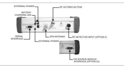
Figure 2-1. S8x0D Test Connector Panel
