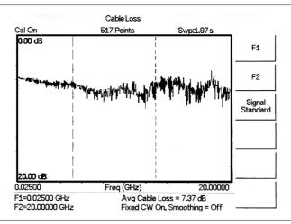
Figure 4-4. Typical Transmission Line Cable Loss Trace
